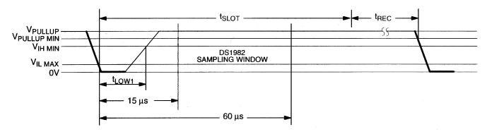
$\begin{array}{l} 60 \ \mu s \leq t_{SLOT} < 120 \ \mu s \\ 1 \ \mu s \leq t_{LOW1} < 15 \ \mu s \\ 1 \ \mu s \leq t_{REC} < \infty \end{array}$
